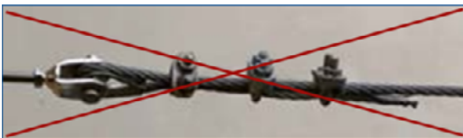
Fig. 15: Rope grip as specified in the former DIN 1142 or EN 13411-5: 2009-02
